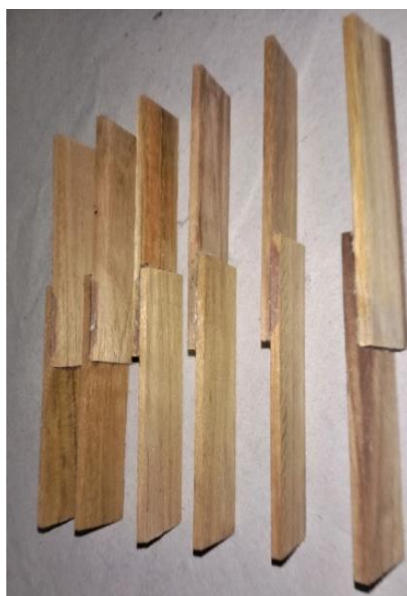
Fig. 2: Preparation of wood blocks for water resistance investigation
