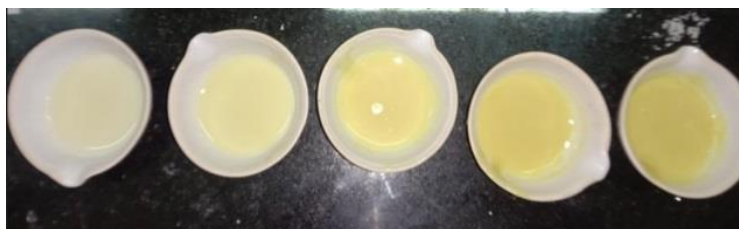
Fig. 1: Different samples of modified sodium silicate with guar gum (2% to 10%)
