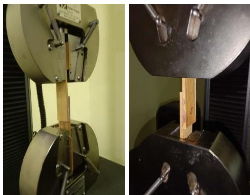
Fig. 3: Tensile strength testing of sodium silicate adhesive on wood blocks
